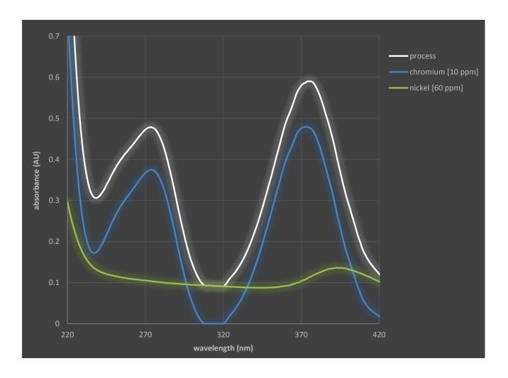
In the figure above, each dot in the process curve represents a single absorbance data point supplied by a photodiode measuring at an integer wavelength. Compiling this rich raw data, the OMA visualizes the total absorbance curve and deconvolutes the absorbance of each metal ion.
